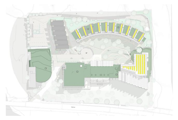
Although PV arrays (in yellow) have been incorporated into the scheme to the maximum extent that roof space allows, and therefore makes a positive contribution to the generation of renewable energy and a real reduction in carbon emissions, the amount of PV array available is in fact unable offset the maximum load to the site and would only assist in minimising carbon emissions.
